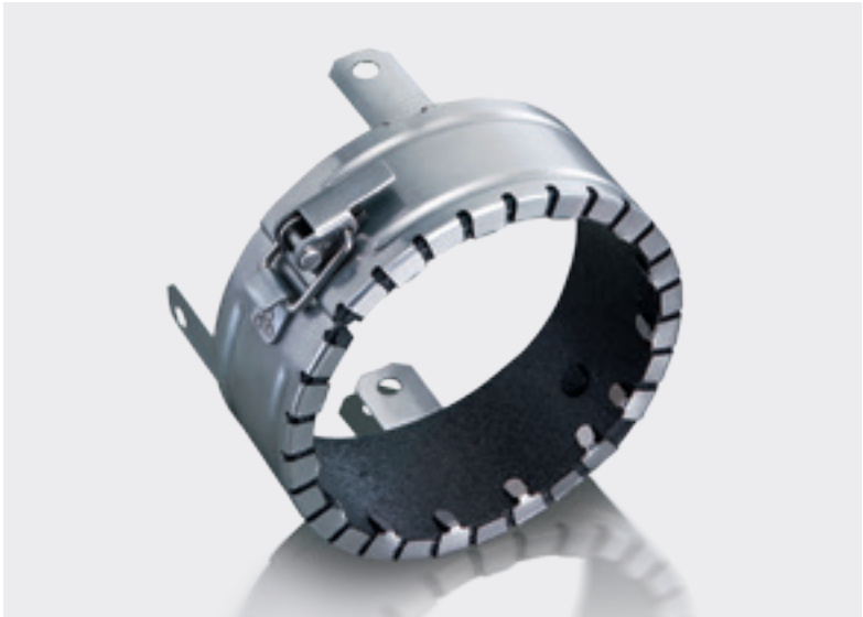
↑ The fire protection sleeve contains an intumescent material which inflates at temperatures of around 150 °C. This inflatable material closes off the feed-through in the ceiling or behind the wall before the fire and smoke can make their way into other rooms or floors.
